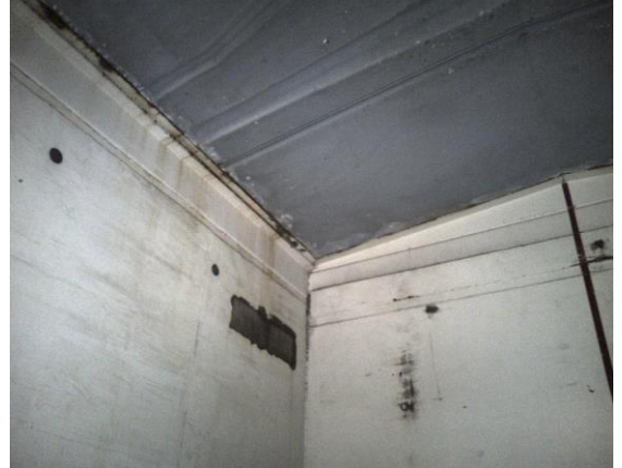
Refrigerated interior railcar roofs refurbished with rust-anode primer Rust-Anode Primer
