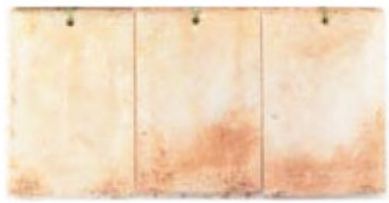
Hot-Dip Galvanized 10000 Hours
